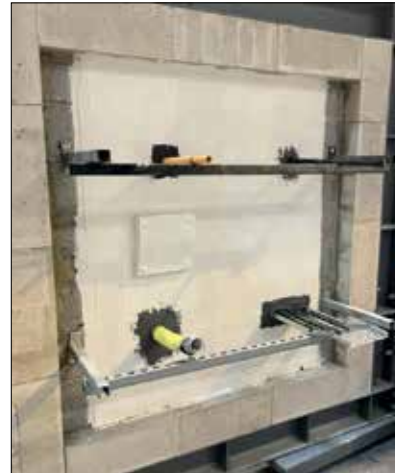
ii. Before the test; external (non-furnace) side
