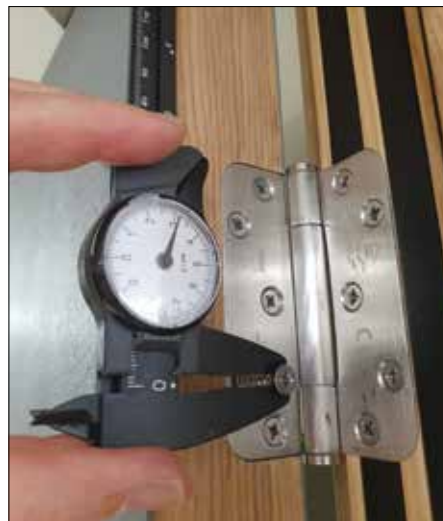
Measuring the diameter of screws using dial calipers during a Type 1 inspection.
