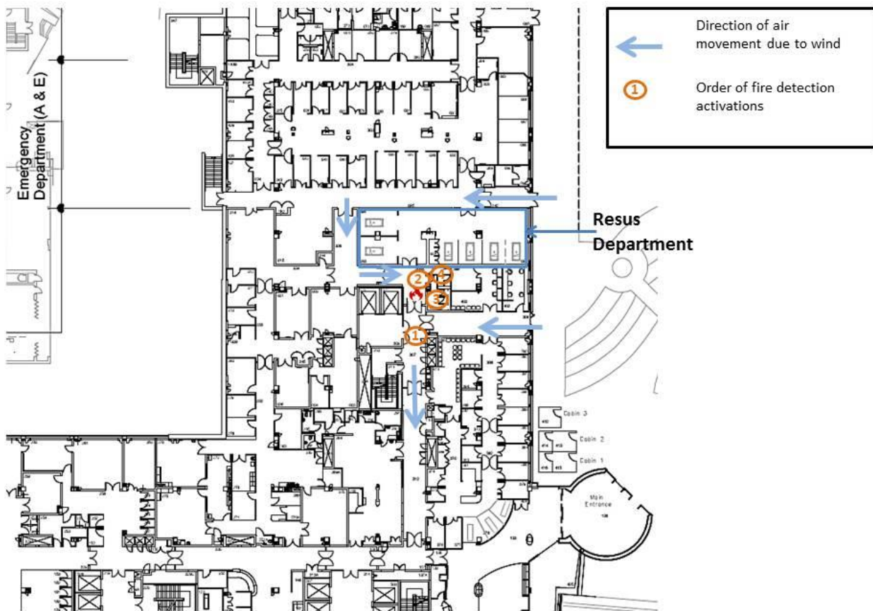
Image / photo 6 - this shows the sequence of detectors operating and air flow into the department drawing the fire initially out of the corridor towards the main corridor. The detector activating closed the fire doors and automatically activated the smoke extract fans
